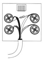
A wall jack with a terminating resistor installed.
