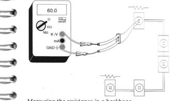
Measuring the resistance in a backbone.
