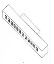
**patch panel:** A wiring distribution block with 12 sets of four RJ11 sockets. A patch panel is used to connect branches that use modular extension cable to a StarController.
