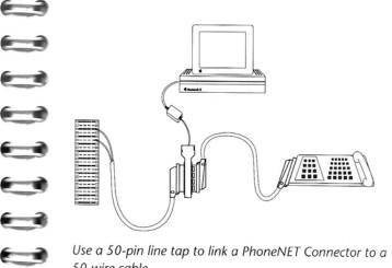
Use a 50-pin line tap to link a PhoneNET Connector to a 50-wire cable
