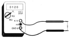
A 120-ohm resistor wrapped around probe ends.
