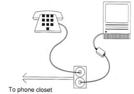
A PhoneNET Connector and telephone plugged into the same wall jack.
