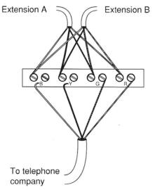
Wiring two extensions into a terminal block.
