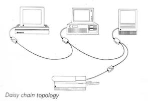
A daisy chain can be constructed quickly and easily, and is a good choice if you want to connect a few devices that are in the same room. A daisy chain is also useful for temporary installations.
