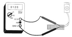
Measuring the resistance in a network branch.
