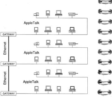
Add an Ethernet backbone to reduce through traffic and improve network performance.
