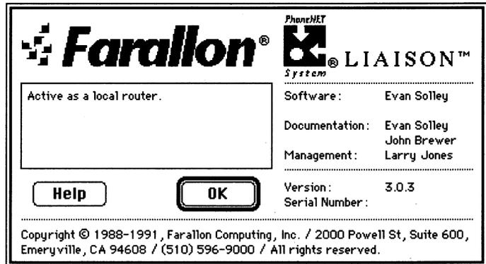
3. To test the full router, go to computers connected to the LocalTalk and TokenTalk networks and make sure you can see the network services on the other side of the router. For example, look for printers in the Chooser.
