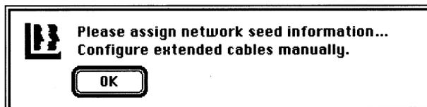
5. Click OK. You need to choose Network Services and manually configure the port that is not selected as the home network of the router. If there is no other router connected to the Ethernet cable, you will also need to assign seed information to the home network too.
