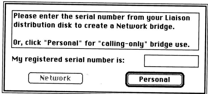
4. Type in the serial number from your Liaison disk. This enables the Network button. (If you do not enter a serial number, clicking the Personal button at this time will limit you to Liaisonet features.) Remember that all copies of Liaison must have unique serial numbers.
