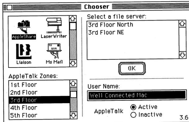
Most importantly, defining zones segments traffic flow. In this example, when the AppleShare icon is selected, only 2 servers (instead of 6) need to reply, cutting back on the traffic generated on the network.
