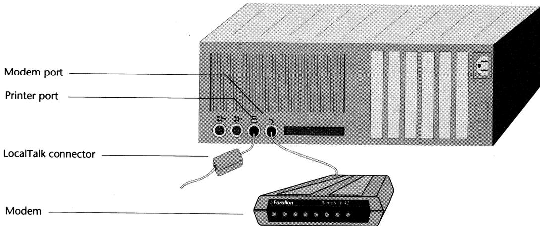
The illustration shows a LocalTalk network cable connected to the printer port. If the answering half-router is on EtherTalk or TokenTalk instead of LocalTalk, the network cable will be attached to the connector on the EtherTalk or TokenTalk adapter.
