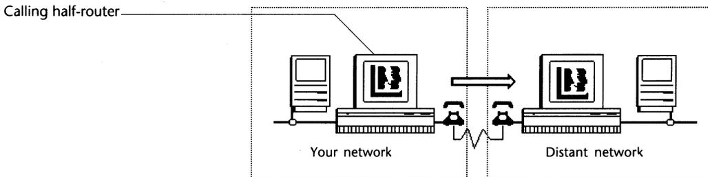
A half-router configuration requires copies of Liaison (including unique serial numbers) and modems on both sides of the dial-up link. The Macintosh on the other side of the link should be configured as an answering half-router. That configuration is explained in the following chapter.
