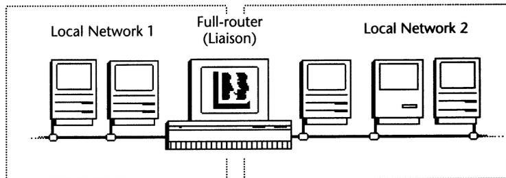
Use Liaison as a full-router to connect two or more networks in the same building or to divide a single overloaded LocalTalk network into smaller, connected ones to speed up network response. You can connect LocalTalk, EtherTalk, and TokenTalk networks together in any combination, and Liaison can support Phase 1 and Phase 2 AppleTalk simultaneously.
