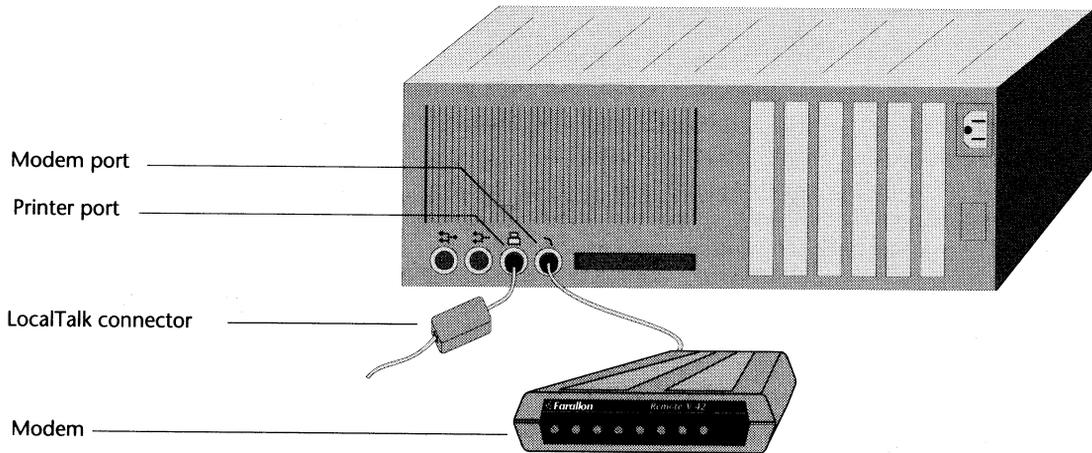
The illustration shows a LocalTalk network cable connected to the printer port. If the calling half-router is on EtherTalk or TokenTalk instead of LocalTalk, the network cable will be attached to the connector on the EtherTalk or TokenTalk adapter.
