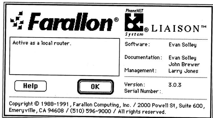
3. To test the full router, go to computers connected to the LocalTalk and EtherTalk networks and make sure you can see the network services on the other side of the router. For example, look for printers in the Chooser.
