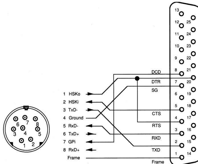
*Preferred Macintosh modem cable. It supports DTR signaling or hardware flow control DCD sensing.*
