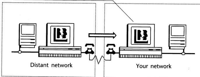
A half-router configuration requires copies of Liaison (including unique serial numbers) and modems on both sides of the dial-up link. The Macintosh on the other side of the link can be configured a calling half-router, personal bridge, or semi-router.
