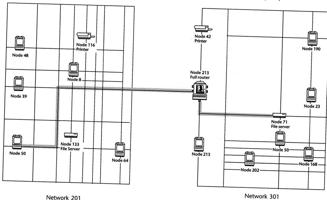
When the AppleShare software at 201/50 sends a data packet to that address, the AppleTalk software at that node determines that 301/71 is not on the immediate network (201) and, therefore, sends it to the full router at Node 213 on Network 301. In this simple internet there is only one router, so the decision is straightforward.
