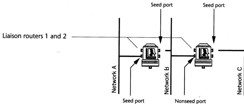
However, Network C has only one router and must get its seeding information from Router 2. Therefore the port connecting Network C to that router must be a seed port.
