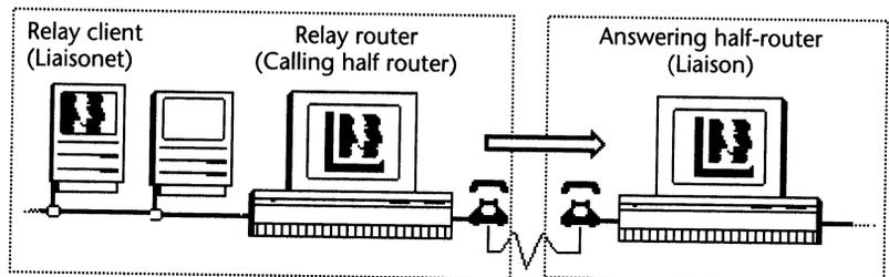
When a user on your network needs to initiate a dial-up connection but does not have a dedicated modem, you can create a **relay client** by installing Liaisonet on that user's computer. The user of the relay client can then select a calling half-router on the network, known in this function as a relay router. The relay router dials the number for the relay client and makes the connection.
