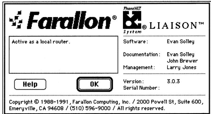
3. To test the full router, go to computers connected to each LocalTalk network and make sure you can see the network services on the other side of the router. For example, look for printers in the Chooser.
