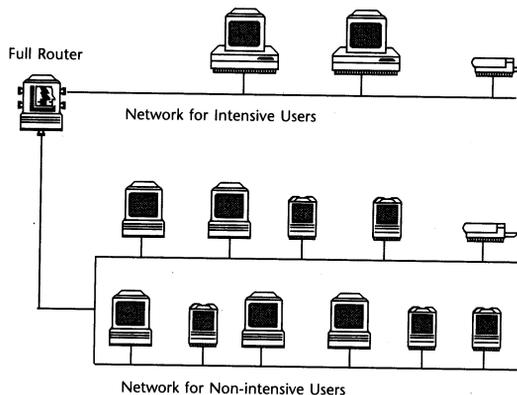
*Dividing an overloaded network into heavy- and light-use networks*
