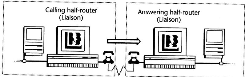
Use Liaison as an answering half-router to receive calls through modems from a distant network. Such a connection makes it possible for users on either side of the dial-up link to access network services (such as electronic mail, print and file servers, and Timbuktu) on the other side of the connection. An answering half-router requires a copy of Liaison and a modem. It can answer calls from a calling half-router, a relay router, a personal bridge, or a semi-router.
