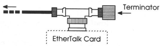
LocalTalk and EtherTalk do not support a continuous loop of cable, nor any T-shaped arrangement of devices. This means that each cable end of each network must be properly terminated with a node for the network to operate correctly.
