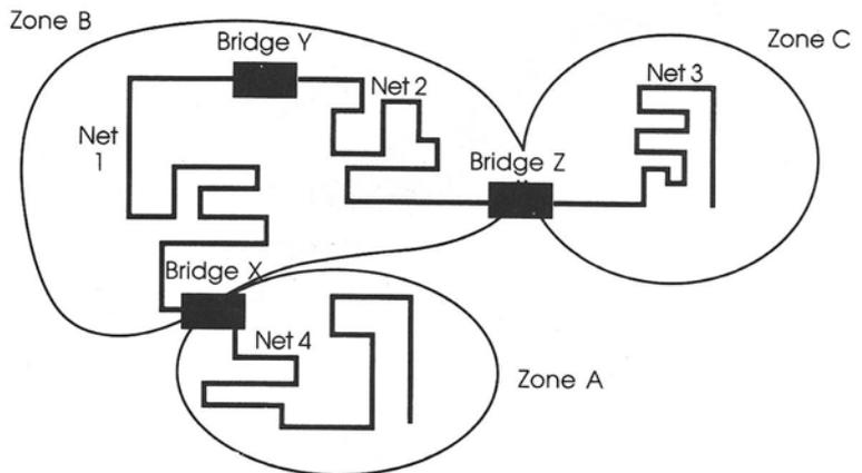
The probable location of the break is now evident. For the administrator's workstation to list networks 4 and 1, yet not 2 or 3, a break must have occurred somewhere at the link between networks 1 and 2.
