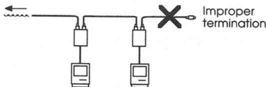
EtherTalk requires a separate terminator at each end of a network segment. EtherTalk is available on various cable media (including twisted-pair and fiber-optic cables) that have different termination requirements. The following represents a terminator for thin Ethernet cabling. Refer to the appropriate installation instructions for the termination requirements of your cable medium.
